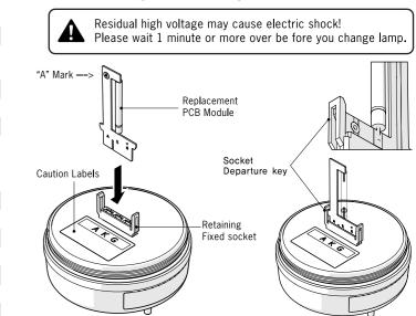
The new lamp should be inserted firmly to match the same signal A K G(or A G K) mark. Printed "A" in circuit and label.
