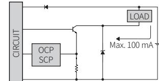
OCP (over current protection, 过电流保护回路), SCP (short circuit protection, 短路保护回路)
