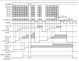
• When the counting value of the channel is arrived at the SV, the alarm output indicator of the channel turns ON. The shaded parts mean flashing the counting value display. Even though the counting value is arrived at the SV, the counting value increases continuously. • Press the [RESET] key to reset the counting value and alarm output indicator of the lowest channel (e.g.: the order of CH 1  $\rightarrow$  CH 15  $\rightarrow$  CH 27) which counting value is arrived at SV.
