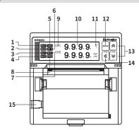
1. Channel 1 alarm (AL1) output indicator: Turns ON when AL1 of input channel 1 operates.
