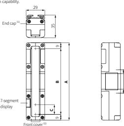
01) When removing the end cap, there is the lamp output terminal (top) or the power supply terminal (bottom).
